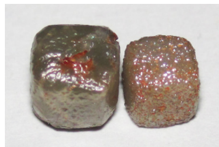
Fibrous diamonds in a cubic morphology
