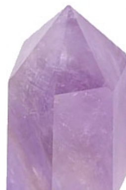
Left: crystal habit of a hexagonal prism with a hexagonal pyramid on top
